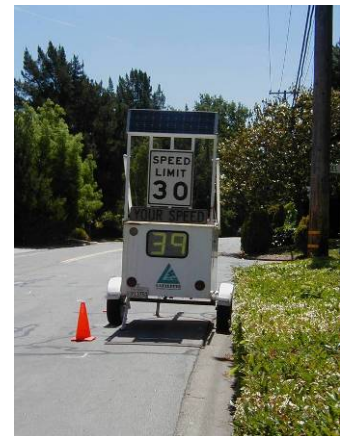
Speed trailer in use.
