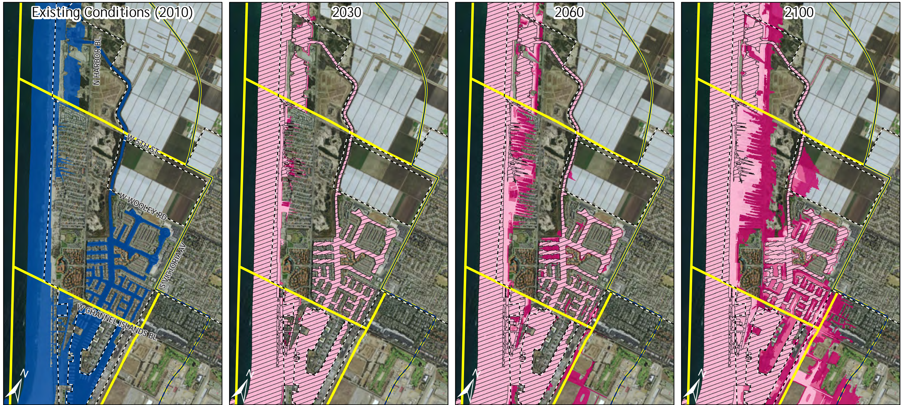
Figure 4.2.4 - Coastal Storm Flood Hazard Zones for Planning Area 2: Oxnard Shores
