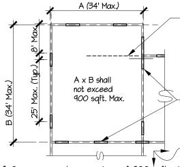
Provide drag struts consisting of blocking with steel strap or joist in line with wall line with strap to top plate of wall
