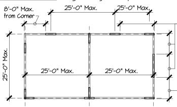
If end distance is greater than 8'-0", an additional shear wall must be added or length added to the shear wall to reduce the distance.
