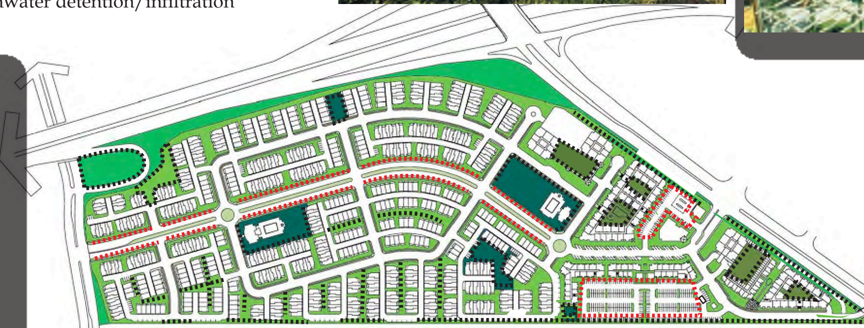
Parks and paseos/corridors can provide stormwater detention/infiltration
