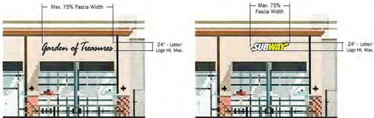
SAMPLE SHOP Tenant ELEVATIONS WITH SIGNAGE
