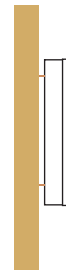
Standard internally illuminated channel letters mounted to a wall or backing, must be mounted 1/2" off the background. Letters may be front, halo or front & halo illuminated.
